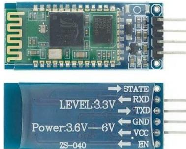
Figura 3. Módulo bluetooth HC-06 (UNIT Electronics, s.f.).
